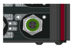
The audio output status indicator next to the M12 connector illuminates when the device is producing sound.
